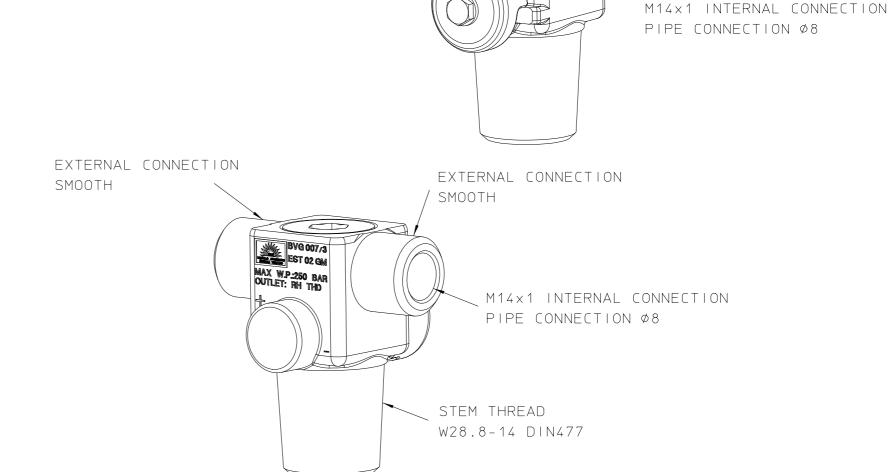
HOMOLOGATION: DGM ITALIA APPROVAL WORKING TEMPERATURE: -40/+85°C WORKING PRESSURE: MAX 260 bar EXTERNAL CONNECTION: SMOOTH
